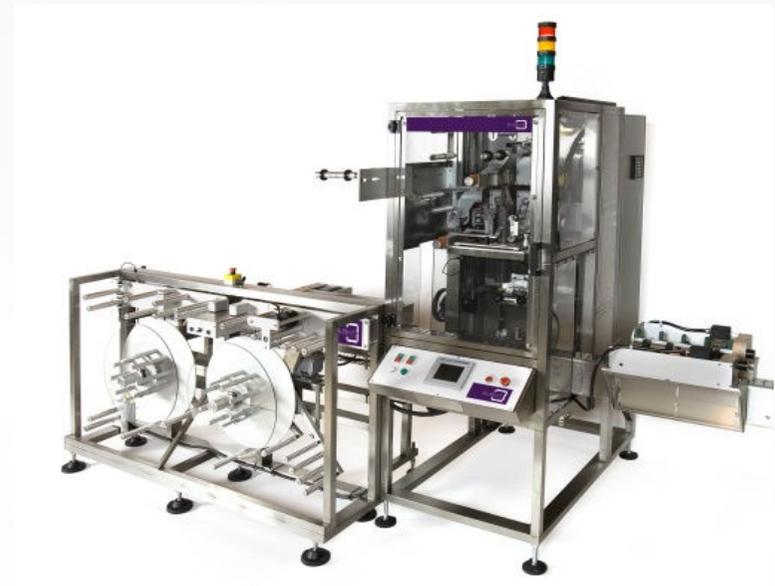
Full body shrink sleeve applicator running at up 800 plus sleeves per minute
